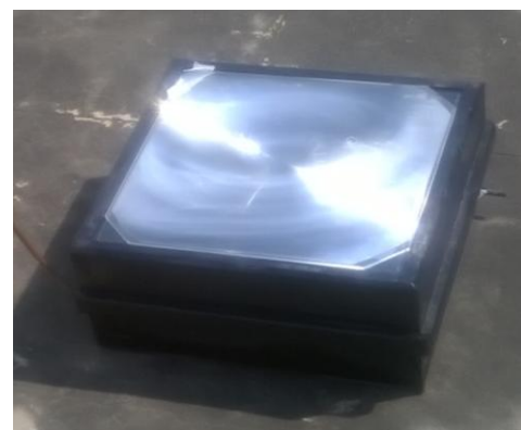
Figure 2 Photograph of FPSWH model with Fresnel lens glazing
