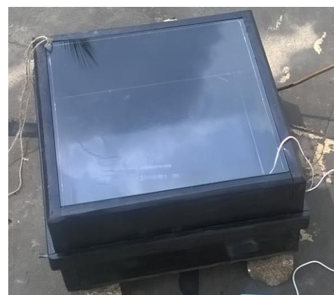
Figure 3 Photograph of FPSWH model with ordinary glazing
