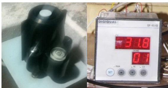
Figure 4 Solarimeter and Universal data logger
